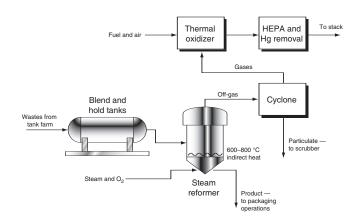
Figure 1. Steam reforming process
