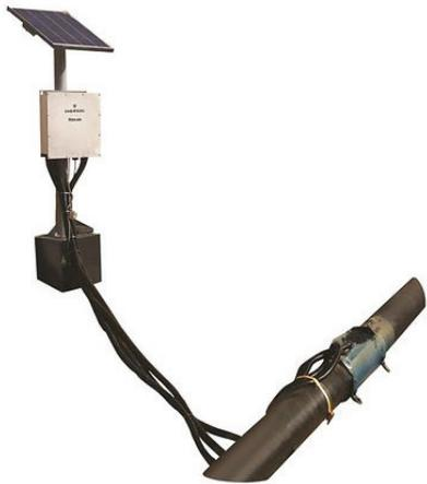
The FSM Area Corrosion Monitor is a non-intrusive solution that can permanently track general and localized metal loss over a pre-defined area in steel pipes, bends and vessels. The multi-pin matrix coverage provides a detailed picture of the pipe area wall thickness, providing a clearer picture of localized corrosion.
