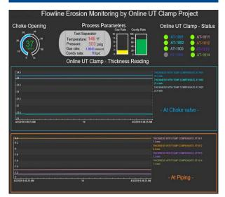
Operators now have HMI graphics indicating thickness measurement trends correlated with the current choke opening and production rate. By watching the historical data, it is possible to see changes in thickness corresponding to sand content and gas velocity.
