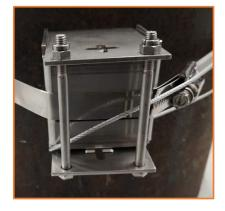
5. ... then through the strap slot of each sensor, the lanyard hole in the sensor head and then into the return hole of the cable lock.
