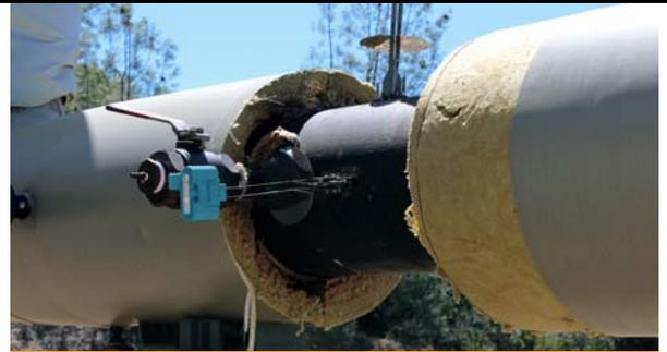
*Operators tried to take manual pipe wall thickness readings using portable ultrasonic measuring devices, but these proved ineffective due to the low repeatability characteristic of the technique, combined with access difficulties.*
