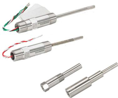
The 68 Series Sensors may be ordered as complete assemblies, by specifying type of sensing element, length, extension, and thermowell. They can be ordered with flying leads, or an enclosure (connection head) with terminal block.
